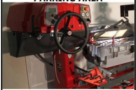
This extra length on the beam (optional) is available to ease the mounting and unmounting of large and heavy cylinder heads on the floating table.
