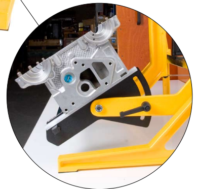
The angle of the head support is adjustable from 0 - 45°
