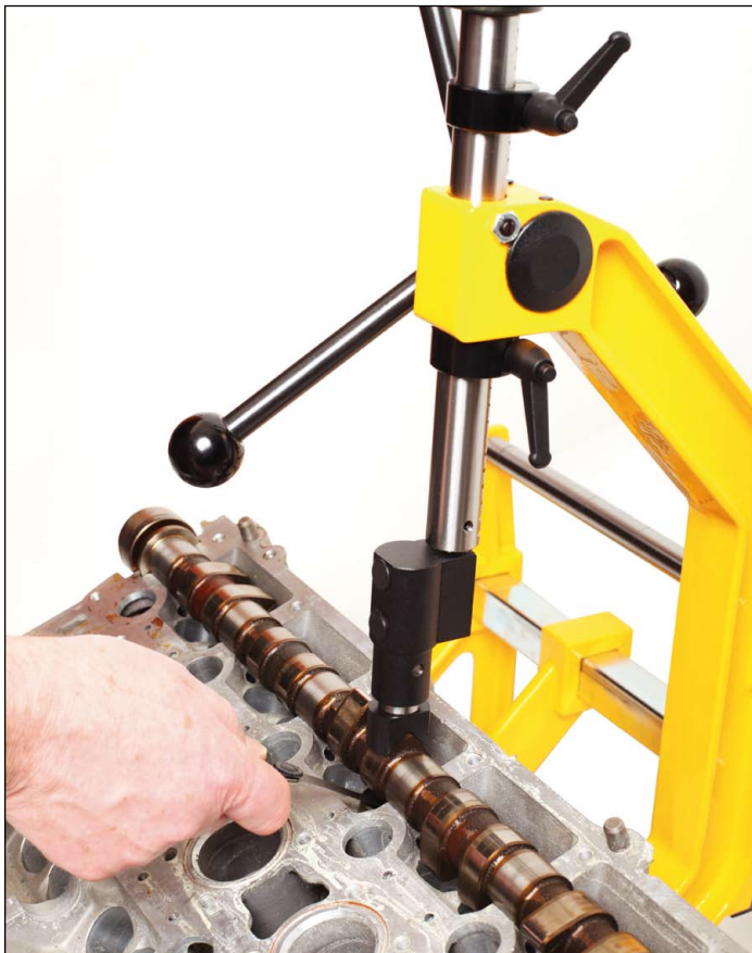
The keepers are easy to remove with the valve keeper magnet.
