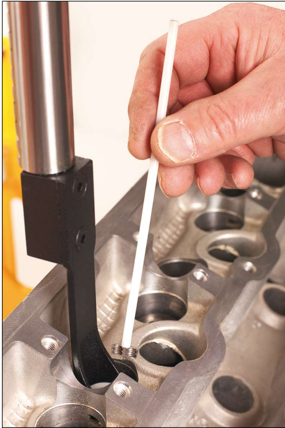
The keepers are easy to remove with the valve keeper magnet.
