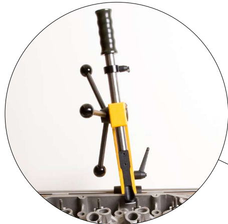
The C-frame is adjustable 25° to both sides for canted valves
